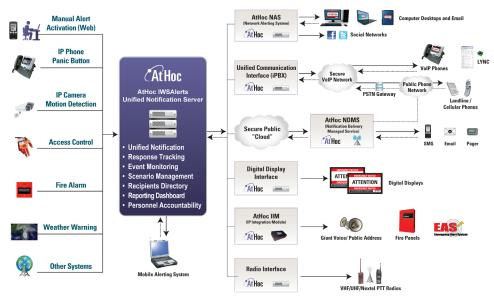
The architecture diagram above shows the role of AtHoc in monitoring events from multiple sources (on left), delivering alerts to multiple devices and capturing responses from individuals (on right)
